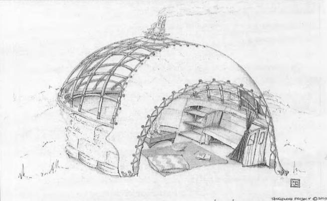
the construction is made of a recycled car tyre base with a straw bale wall covered by timber frame structure and canvas conopy. It is embbeded in a existing grass mound.
